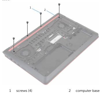
5 Lift the computer base and, using a plastic scribe, release the palm-rest assembly from the computer base
